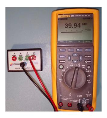
Be sure operator is grounded during the tests so the 50/60 Hz noise will not affect the Tester Verification Unit operation of the device.
