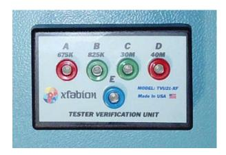
(1) Use a calibrated DMM to verify the resistances are within 10% of the stated values.
